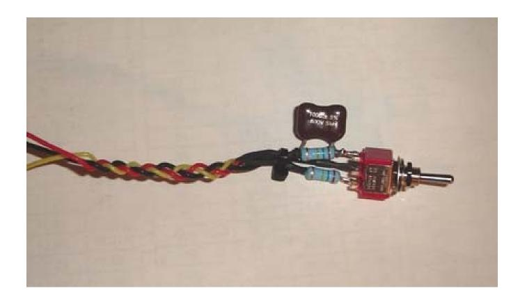
Then I installed the switch into place on the front panel, using some flat washers between the standard switch washers and the panel because of the larger hole, and ran the wires to the board and soldered them to the turrets. The two wires with the resistors go to the two outer turrets that also contain the coupling caps. The wire from the center terminal goes to the center turret, the empty one. And it looks like this: (see photo on next page)
