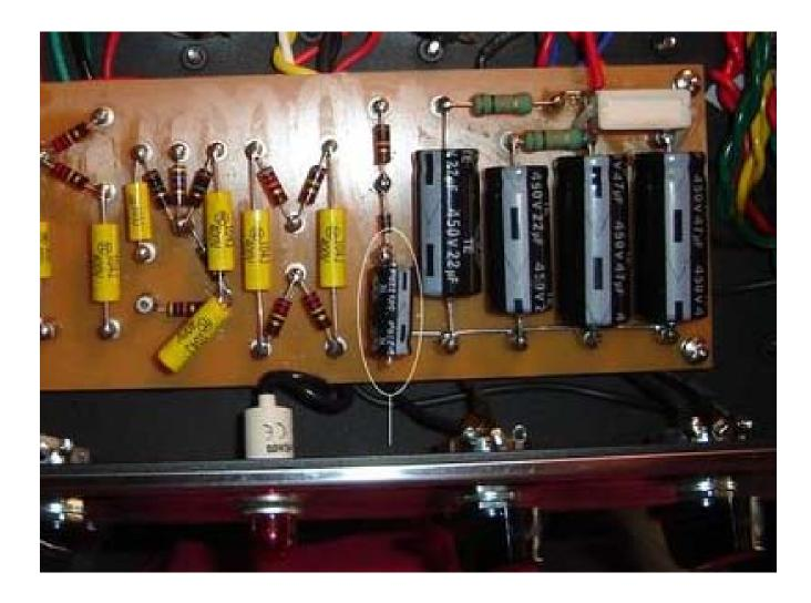
1. First thing to do is to remove the capacitor, but be careful, you'll need to put it back later. Heat the turrets until the solder melts and gently pull the leads out and set the cap aside where it will be safe for when you need it later.
