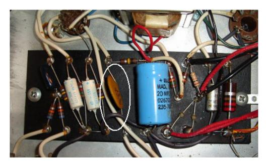
To remove the cap just heat the eyelet that each lead is soldered to until the solder melts and you can pull the lead loose with a pair of small pliers.
